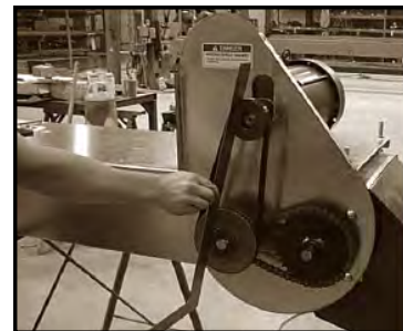
Lay a straightedge across pulley faces
