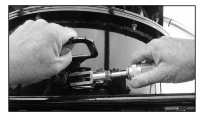
To fine tune the seed flow rate, loosen the nut on the bottom part of the adjustment rod. The rod can then be threaded in and out for minor seed flow adjustments.
