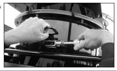
To adjust the seed flow, Move the coupler to a different notch on the adjustment rod. The more notches exposed, means more seed is allowed through the gate.
