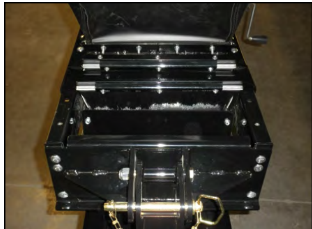
Bottom clean-out cover removed
