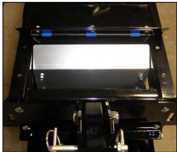
Bottom clean-out cover removed
