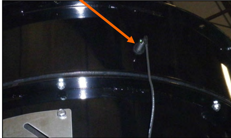
SMW HOPPER PROXIMITY SENSOR
