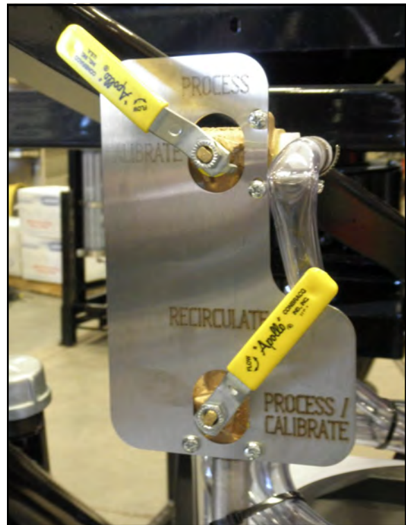
Right Tank Source Valve
