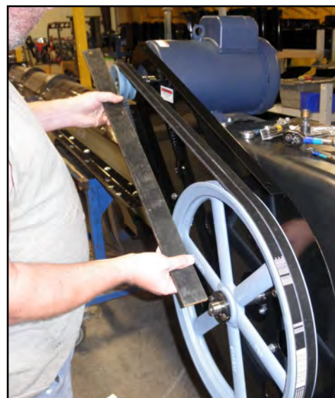
Lay a Straightedge Across Pulley Faces
