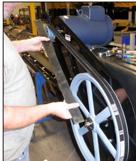
Lay a Straightedge Across Pulley Faces
