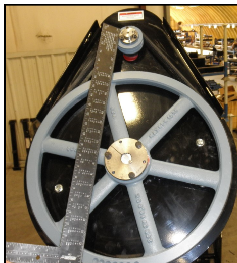
Lay a straightedge across pulley faces
