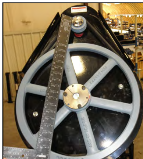
Lay a straightedge across pulley faces
