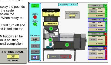
10. Once the data has been saved, the operator may access the report from the UTILITIES screen by selecting the REPORTS button in the lower left corner. If a printer is plugged into an Ethernet port on the bottom of the control panel, the PRINT button may be pressed to print the data for the customer's records.
