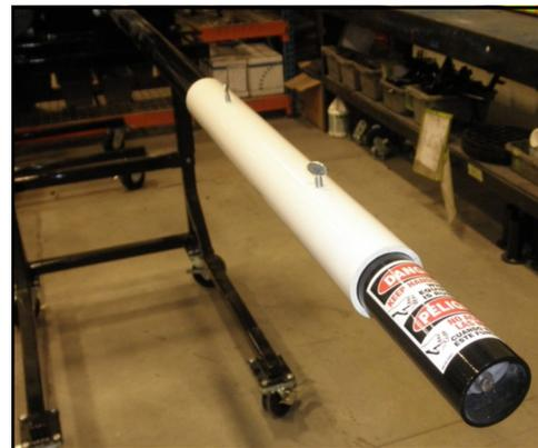
*Calibration Sleeve at end of Auger Tube*
