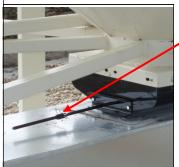
Move the position of the collar along this rod to adjust the flow of seed through the bin slide
