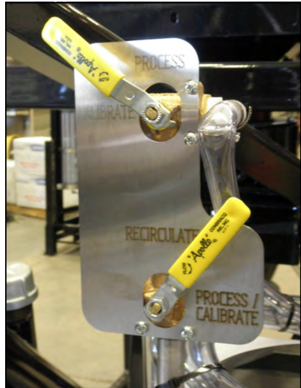
Right Tank Source Valve
