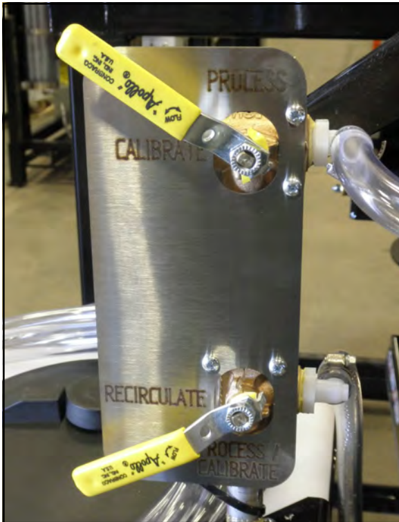
Left Tank Source Valve
