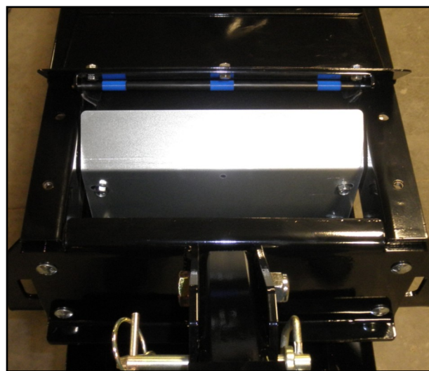
Bottom clean-out cover removed
