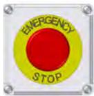
There is one Emergency Stop push buttons located on the LX Series Seed Treater, which is located on the main control. Actuators of emergency stop shall be colored RED. The background immediately around the device actuator shall be colored YELLOW. The actuator pushbutton-operated device shall be of the palm or mushroom head type.
