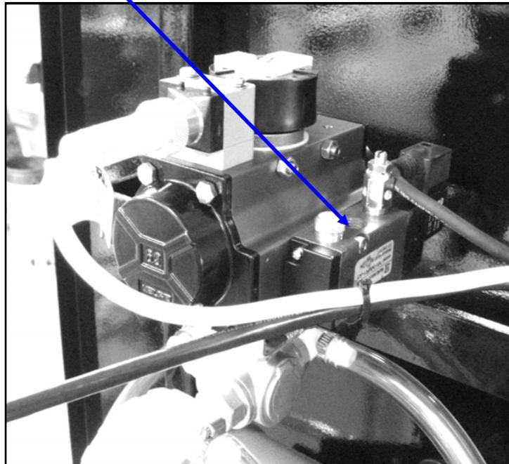
10. The proximity switches which are sent with the treater will need to be installed in the overhead supply hopper. Below is a picture of a LP4000 which includes an overhead hopper that is built by USC. The picture illustrates where the proximity switches need to be mounted.
