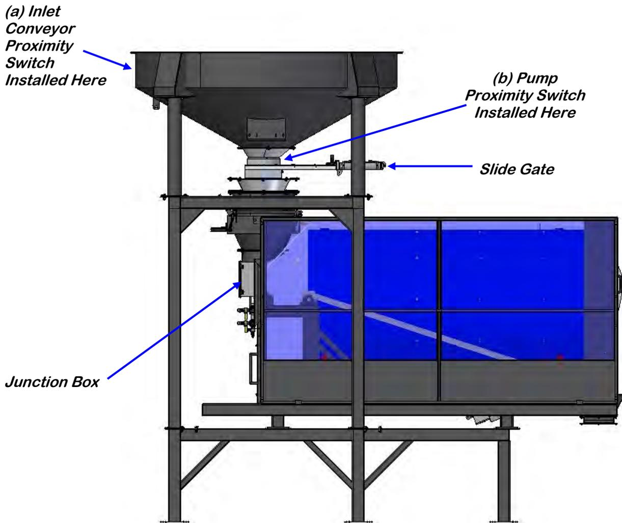
13. Have a certified electrician provide power to the seed treating system. Provide convenient shutdown switches, comply with local electrical codes and ensure that the system is properly grounded and bonded. The USC system must be connected to the same electrical requirements as specified in the main control panel on the power requirement tag, or the electrical schematic shipped with the piece of equipment. This will power the entire USC system.
