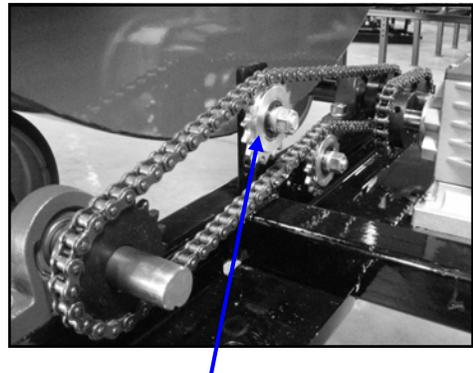
*Use this sprocket to tighten chain*
