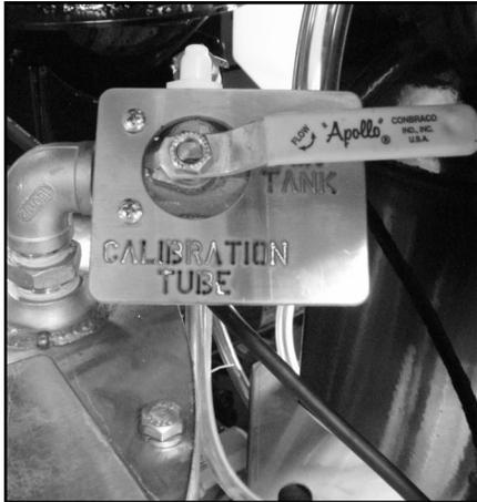
*Pump #1 pumping liquid into the top of the mix tank when Seed Treatment Valve is in Calibrate.*
