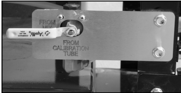
Drawing chemical from the bottom of the Mix Tank
