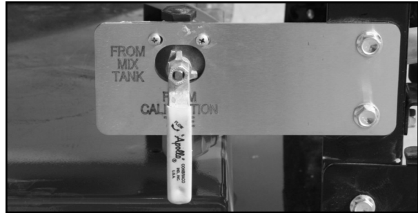
Drawing chemical from the bottom of the Calibration Tube
