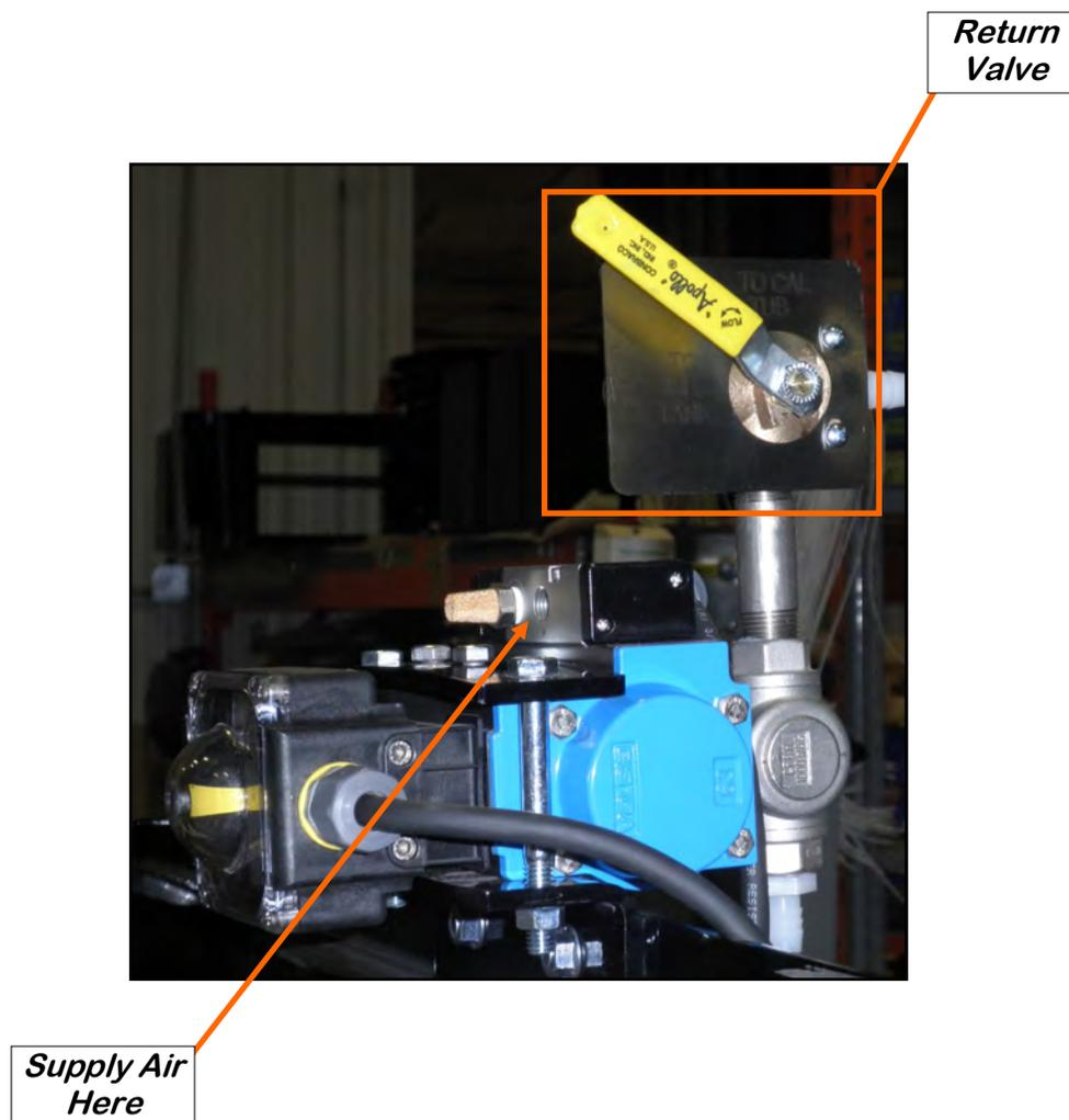
**AIR ACTUATED 3-WAY VALVE:** This valve is controlled from the touch screen and will automatically actuate during normal operation. An internal spring holds the valve in the recirculation position so that when the valve is not actuated, the chemical will be directed to flow back to the Mix Tank. When the valve is actuated, the supplied air pressure will override the spring and move the valve to the PROCESS position. Chemical flow will then be directed towards the treater's atomizer chamber.
