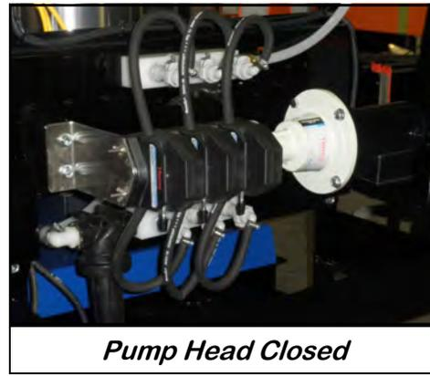
If a very low rate is needed, a section of tubing can be removed to force the pump motor to run at a higher speed. This allows for a more consistent flow rate. When removing the tubing, uncouple it from the manifold (below, right). If the tubing is unclamped from the pump head but left coupled in the manifold (below, left), the pump will suck air and cause flow rates to be very inconsistent.
