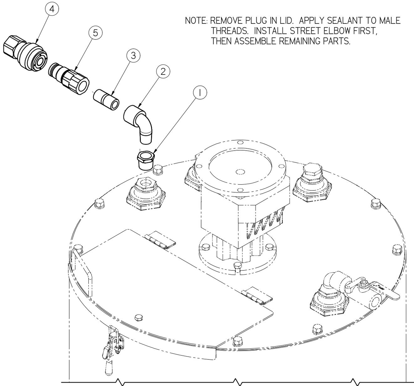
NOTE: REMOVE PLUG IN LID. APPLY SEALANT TO MALE THREADS. INSTALL STREET ELBOW FIRST, THEN ASSEMBLE REMAINING PARTS.
