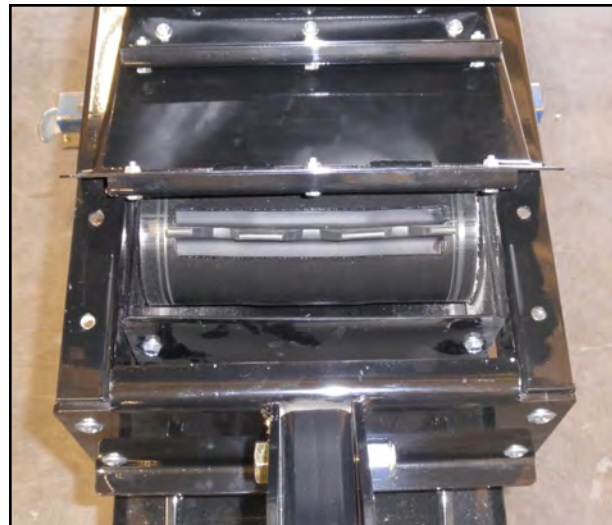
Bottom clean-out cover removed
