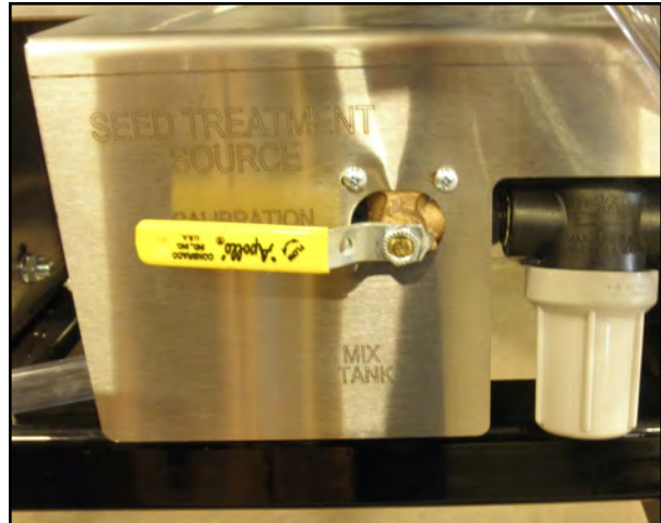
Pump #1 Drawing from bottom of Calibration Tube
