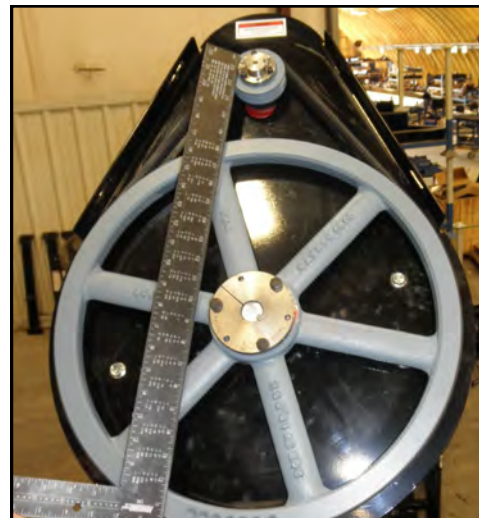
Lay a straightedge across pulley faces
