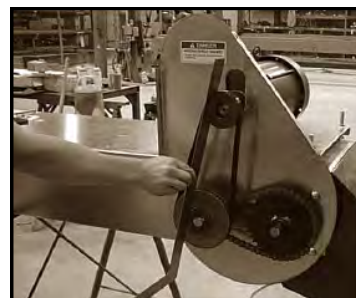
Lay a straightedge across pulley faces
