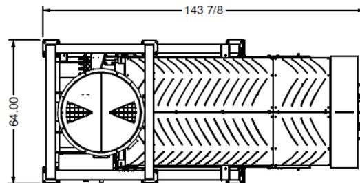
LPV LIW for Bulk Site Systems (required weigh hopper not shown)
