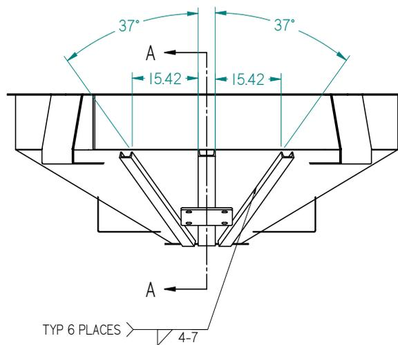
STITCH WELDS MUST START AND STOP 1" FROM ENDS TO PREVENT CRACKING
