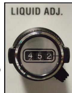
**EXAMPLE:** The seed treatment slurry rate is 4 ounces per cwt.
