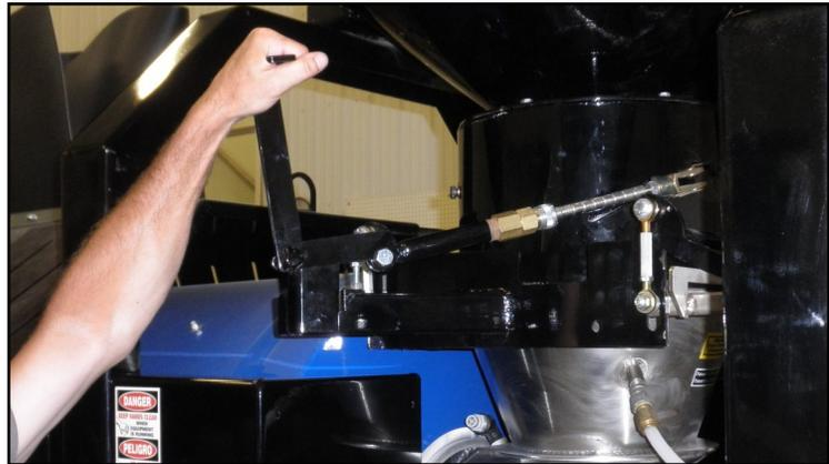
Regulate the amount of seed flowing through the seed treater by using the spring-loaded coupler and moving it to a different notch. The more notches exposed, the higher the seed flow.
