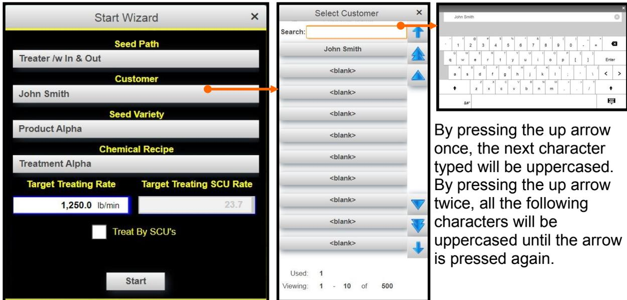
By pressing the up arrow once, the next character typed will be uppercased. By pressing the up arrow twice, all the following characters will be uppercased until the arrow is pressed again.
