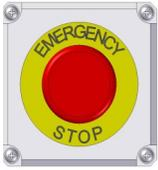
There is an Emergency Stop push button on all LPV and LPX Seed Treater which is located on the Treater Control Panel. The LPX Automated Treater has an additional Emergency Stop pushbutton on the Main Control Panel. Actuators of emergency stop shall be colored RED. The background immediately around the device actuator shall be colored YELLOW. The actuator pushbutton operated device shall be of the palm or mushroom head type.
