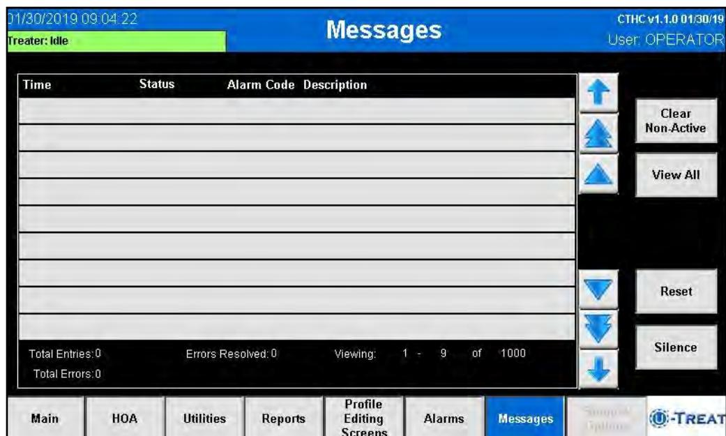
**1. CLEAR NON-ACTIVE:** The message status will change to Acknowledged once an alarm condition has been resolved and the Reset button has cleared the alarm. Pressing this button will clear all alarms with the status of acknowledged.
