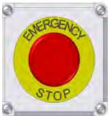
There is an Emergency Stop push button on all CTHC 3000 Seed Treaters which is located on the Treater Control Panel. Actuators of emergency stop shall be colored RED. The background immediately around the device actuator shall be colored YELLOW. The actuator pushbutton operated device shall be of the palm or mushroom head type.
