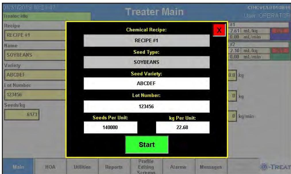
4. As the seed is being treated, the main screen will display the box weight and the liquid flow rate. If the system needs to be stopped for a moment, the Pause button may be pressed to temporarily stop the process. When ready to begin again, press the Continue button on the Continue / Terminate popup screen.
