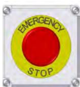
There is an Emergency Stop push button on all CTHC 3000 Seed Treaters which is located on the Treater Control Panel. Actuators of emergency stop shall be colored RED. The background immediately around the device actuator shall be colored YELLOW. The actuator pushbutton operated device shall be of the palm or mushroom head type.
