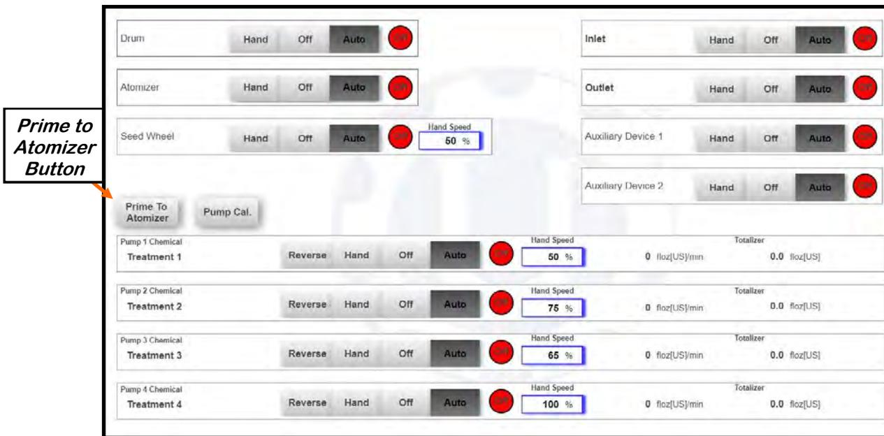
3. Return to the main screen and press the Start Setup button. Press the gray buttons to change the Seed Path, Customer, Seed Type, or Recipe fields. Press Start to begin the run. The atomizer, drum, and any inlet conveyors will turn on. Feed the system with seed. When the proximity switch detects seed, a timer will count down the number of seconds the start delay was set for. When that time elapses, the slide gate will open or the seed wheel will turn on depending on your system.
