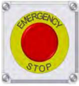
There is an Emergency Stop push button on all LPV and LPX Seed Treater which is located on the Treater Control Panel. The LPX Automated Treater has an additional Emergency Stop pushbutton on the Main Control Panel. Actuators of emergency stop shall be colored RED. The background immediately around the device actuator shall be colored YELLOW. The actuator pushbutton operated device shall be of the palm or mushroom head type.
