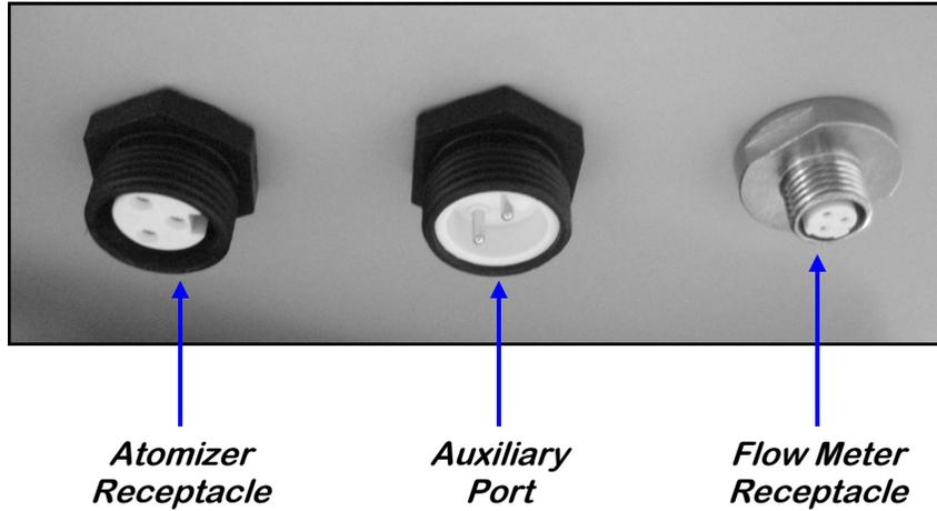
**Atomizer Receptacle:** This receptacle is where the motor that runs the atomizer is plugged in to. The atomizer can be unplugged so it can be removed for service and clean-up.
