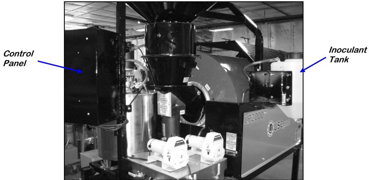
2. Release the red-handled clamp and remove the small shipping bolt. Also loosen the two 5/16" bolts, located towards the front of the atomizer. This holds the top atomizer flange tight against the adjustable seed gate flange (below right).
