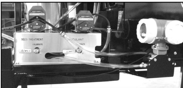
12. Connect any conveyors into the seed treater control panel. Ensure that the conveyors being used are the same power ratings as the seed treater.
