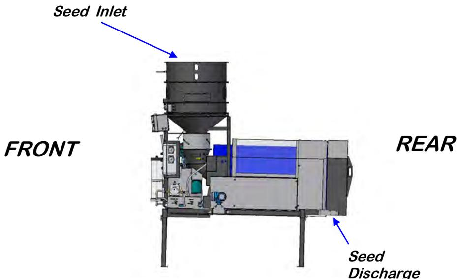
4. Remove any boxes and the front leg from the drum of the treater.
