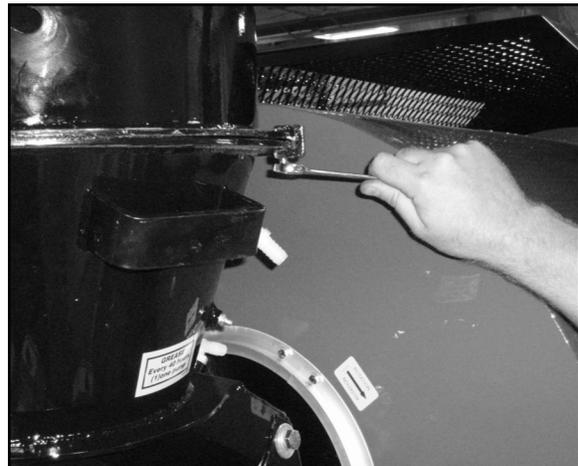
3. Slide the atomizer straight back and drop down to access the atomizer head and bearing (below). To completely remove the housing from the treater, unplug the motor from the control panel and disconnect the treatment lines.
