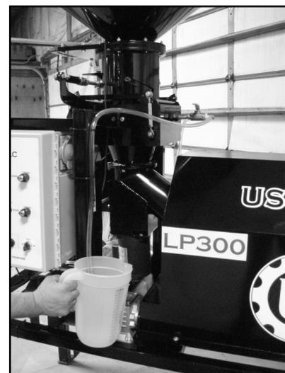
**Calibrating pump with measuring cup.**
