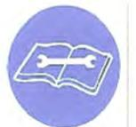
**Mandatory Read Manual Action Symbol.** (I.S.O. format) This symbol instructs personnel to read the Operators Manual before servicing or operating the equipment.
