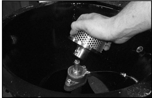
4. The atomizer head is threaded together. Unscrew the head for better access to cleaning.
