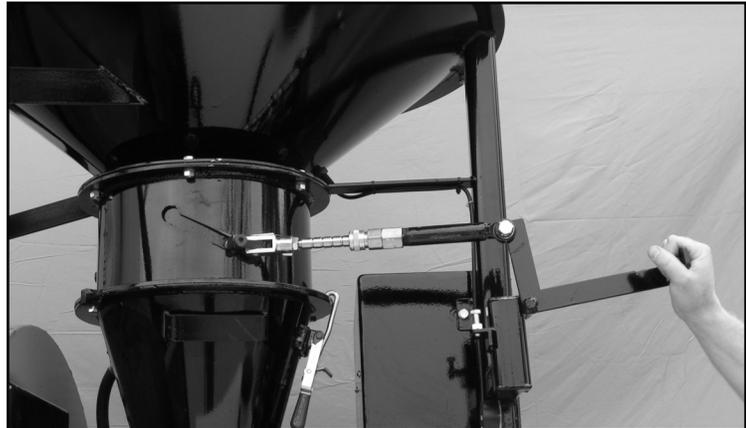
When the black lever is pushed up, the seed gate is in the open position, and seed will flow through
