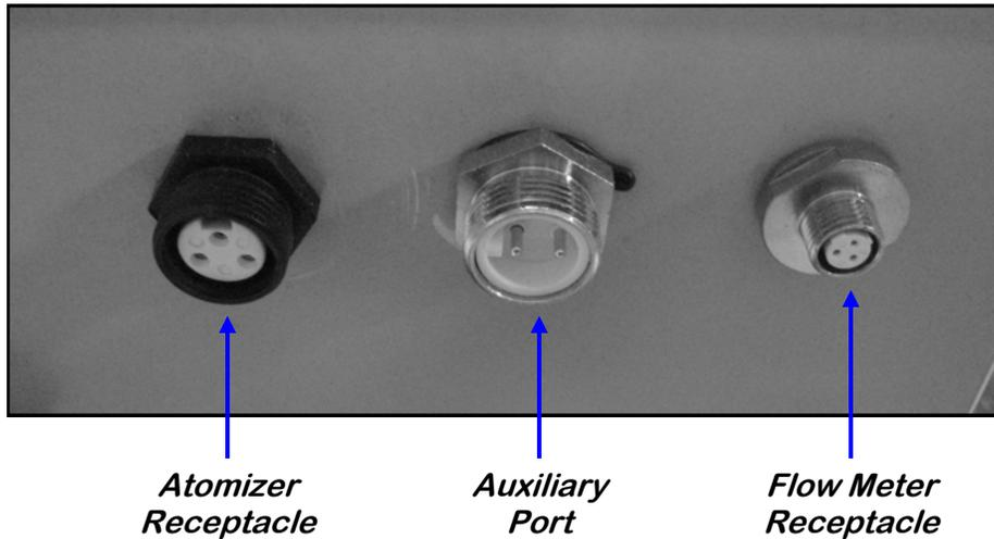
**Atomizer Receptacle:** This receptacle is where the motor which runs the atomizer is plugged in to. The atomizer can be unplugged so it can be removed from the machine for maintenance.
