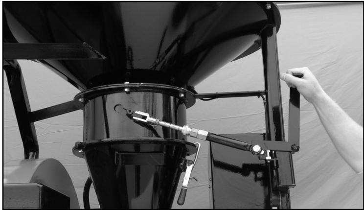
Regulate the amount of seed flowing through the seed treater by using the spring-loaded coupler and moving it to a different notch. The more notches exposed, the higher the seed flow.
