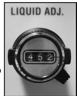
**EXAMPLE:** The seed treatment slurry rate is 4 ounces per cwt.
