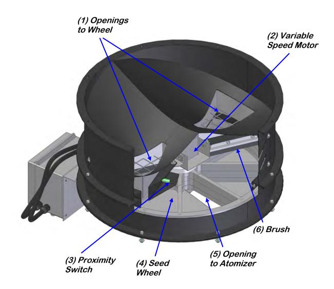
*<u>1. Openings to Wheel</u>*: This is where the seed is dispensed into the wheel pockets.
