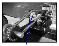
Use this sprocket to tighten chain
