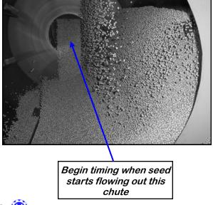
The Illustration below shows how seed passes through the atomizing chamber. The blue represents treatment being dispensed to the seed as it passes through the chamber. After the seed passes through the atomizer, it goes into the drum where the coating process is completed.
