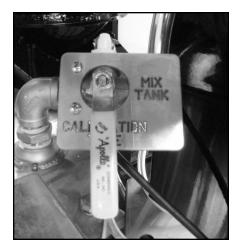
Pump #1 pumping liquid into the top of the calibration tube when Seed Treatment Valve is in Calibrate.
