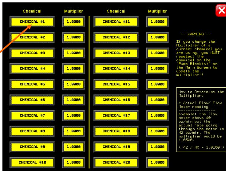
**3. EDIT CHEMICAL NAMES (CONTINUED):** This screen also allows the operator to recalibrate the flow meter by adjusting the multiplier for each chemical.
