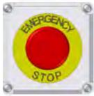
There are two Emergency Stop push buttons on the LX Series Seed Treater, which are located on the main control panel and the treater junction box. Actuators of emergency stop shall be colored RED. The background immediately around the device actuator shall be colored YELLOW. The actuator pushbutton-operated device shall be of the palm or mushroom head type.
