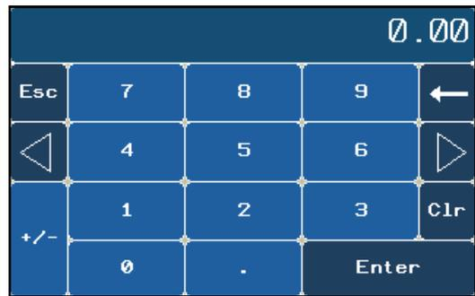
**8. Atomizer Percent Speed:** When this button is pressed, a numeric touch pad (right) will appear to allow the operator to manually adjust the speed of the atomizer.
