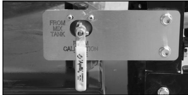
*Drawing chemical from the bottom of the Calibration Tube*
