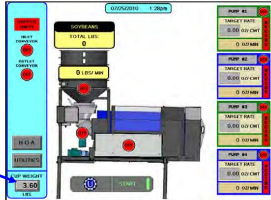
8. Press the Utilities button on the main screen to advance to the utilities screen. Enter in the Target Treating Rate in pounds per minute. Also at this time fill in all other parameters on this screen. Below is a screen shot of the utilities screen with typical numbers to use when beginning to treat.
