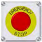
There are two Emergency Stop push buttons on the MX Series Seed Treater, which are located on the main control panel and the treater junction box. Actuators of emergency stop shall be colored RED. The background immediately around the device actuator shall be colored YELLOW. The actuator pushbutton-operated device shall be of the palm or mushroom head type.
