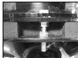
(B): Install the 3/8" flange nut to the alignment bolt.
