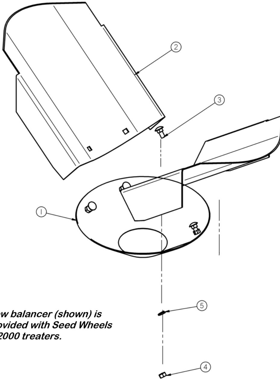
*The flow balancer (shown) is not provided with Seed Wheels for LP2000 treaters.*
