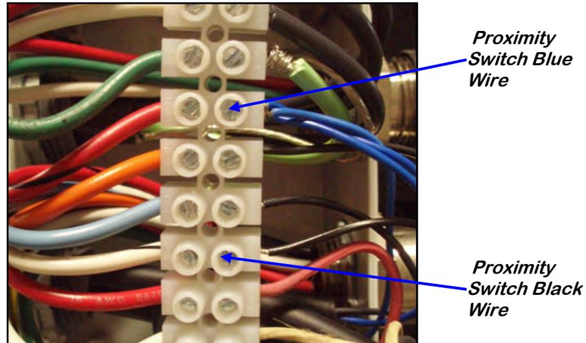
4. The 4-wire cord coming out of the bottom of the seed wheel control panel wires into the seed treater panel.
