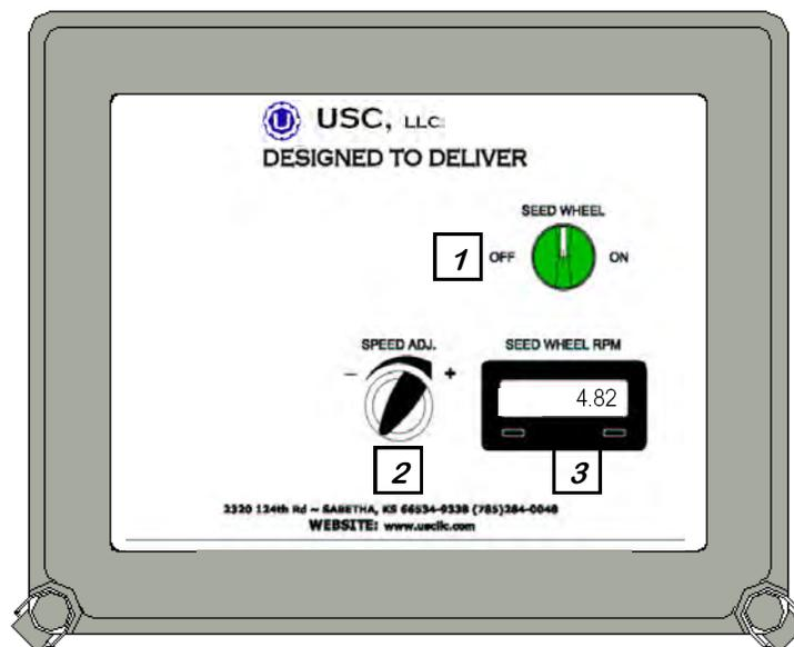
**1. Seed Wheel:** Allows the operator to turn the seed wheel on or off.
