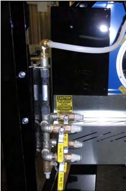
7. For LPX, LX and MX treaters, attach the chemical tubing from the pump stand(s) to the atomizer plumbing on the seed treater (left). For all other treaters additional tubing can be added or removed to accommodate your set-up.
