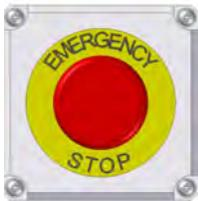
There are three Emergency Stop push buttons on the Portable LPV Seed Treater. One is located on the I / O control panel mounted on the side of the treater, and one each on the Treater Control and Main Control Panels mounted on the side of the trailer. All Actuators of emergency stop shall be colored RED. The background immediately around the device actuator shall be colored YELLOW. The actuator pushbutton operated device shall be of the palm or mushroom head type.
