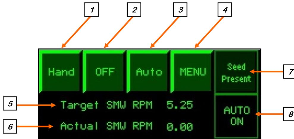
**1. HAND BUTTON:** Pushing this button will start the system in the manual mode of operation.
