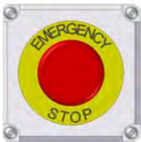
There is an Emergency Stop push button located on the Main Control Panel. Actuators of emergency stop shall be colored RED. The background immediately around the device actuator shall be colored YELLOW. The actuator pushbutton operated device shall be of the palm or mushroom head type.
