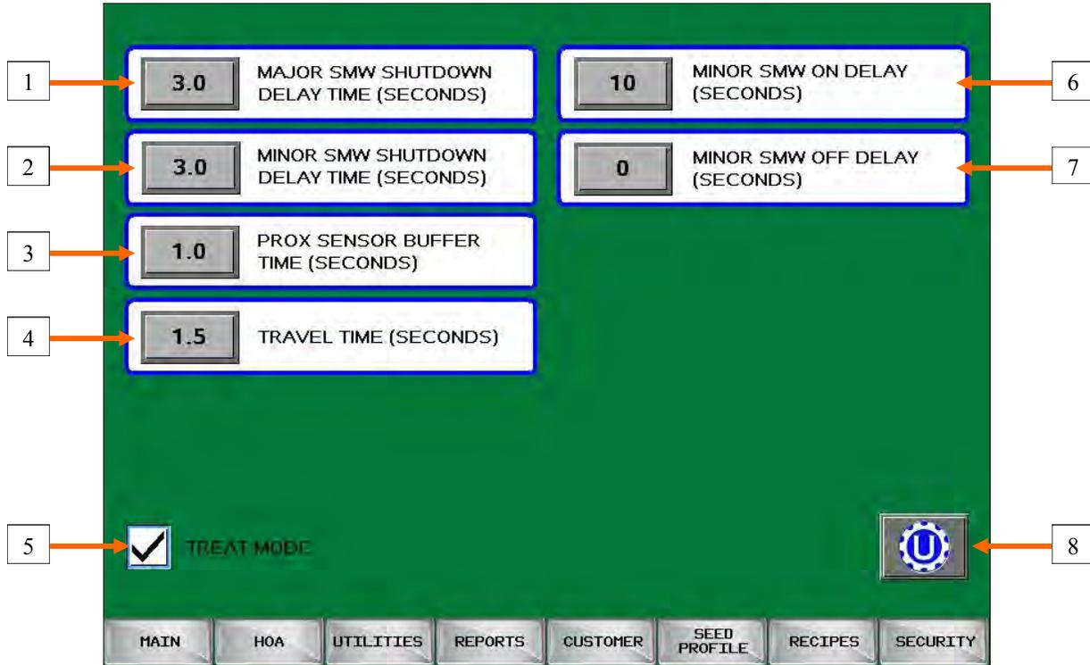
**NOTICE** When buttons 1 - 4, 6 and 7 are pressed, a numeric touch pad (right) will appear allowing the operator to enter in a number for that particular parameter.
