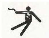
**Electrocution Hazard Symbol.** This symbol indicates that an electrocution hazard exists. Serious injury or death could result from contacting high voltage.
