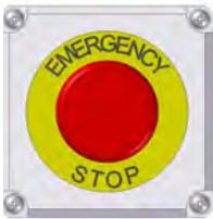
There is an Emergency Stop push button on the Seed Conditioner located on the Main Control Panel. Actuators of emergency stop shall be colored RED. The background immediately around the device actuator shall be colored YELLOW. The actuator pushbutton operated device shall be of the palm or mushroom head type.
