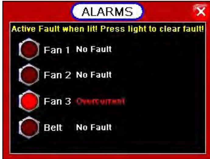
When an alarm is active, the indicator will be illuminated as shown above on Fan 3 and the alarm text will flash red and white. When the alarm is resolved the text will remain white and the light will remain lit until the operator presses it to clear the fault.
