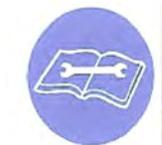
**Mandatory Read Manual Action Symbol.** (I.S.O. format) This symbol instructs personnel to read the Operators Manual before servicing or operating the equipment.
