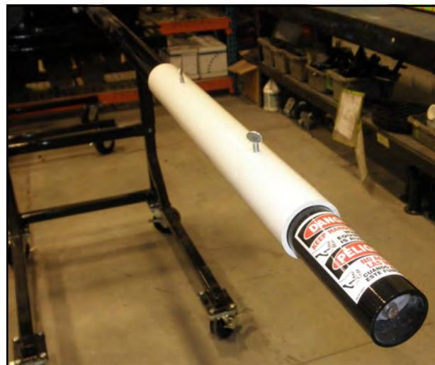
*Calibration Sleeve at end of Auger Tube*
