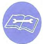
**Mandatory Read Manual Action Symbol.** (I.S.O. format) This symbol instructs personnel to read the Operators Manual before servicing or operating the equipment.
