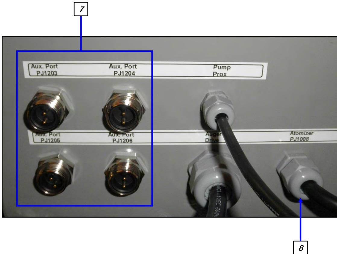
7. Connect the communication cable from the pump stand(s) to any of the four two wire connectors on the bottom of the control panel (PJ1203 - PJ1204).
