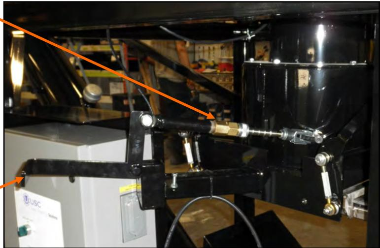
When the black lever is pushed up, the seed gate is in the open position, and seed will flow through.
