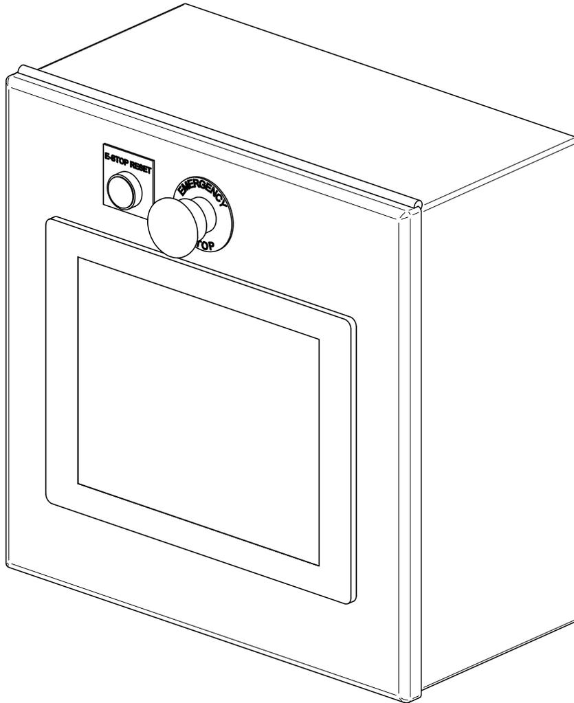
There is an optional remote Automated Treater Control Panel. It allows the operator to run the treater from up to 50 feet away. If it is ordered with the treater, it will come with the HMI operation screen already installed. If it is added later as an upgrade, the HMI will be removed from the original Control Panel and installed in the remote panel. A plug is included in the kit to plug the hole in the main panel after the HMI is removed. The remote panel comes with a 10 foot power cord.
