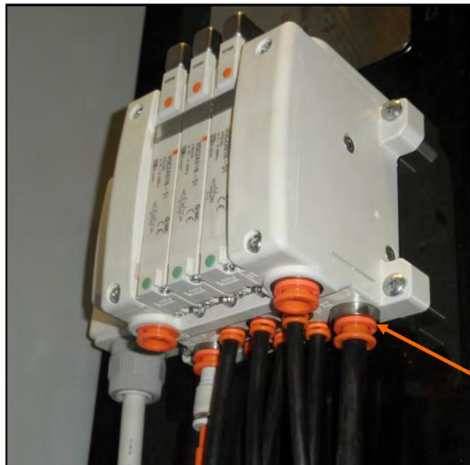
13. Run two 1/4 inch lines from A&B WYE TO POWDER UNIT to the “Y” fitting on the back of the control panel.
