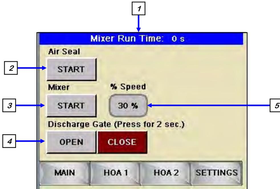
**1. MIXER RUN TIME INDICATOR:** Informs the operator of the amount of time in seconds the mixer has been running after the START button has been pressed. If the STOP button is pressed while a batch is in process, the timer will stop until the system is re-started.
