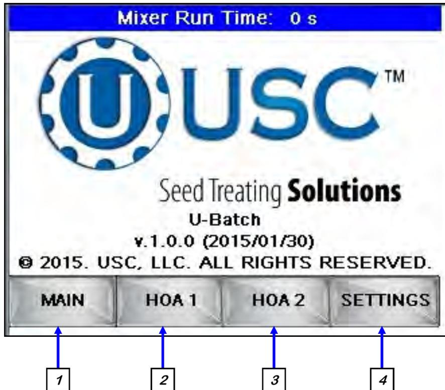
**1. MAIN SCREEN BUTTON:** Pressing this button returns the operator to the MAIN screen.
