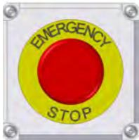
There is an Emergency Stop push button on the Batch Coater which is located on the Main Control Panel. Actuators of emergency stop shall be colored RED. The background immediately around the device actuator shall be colored YELLOW. The actuator pushbutton operated device shall be of the palm or mushroom head type.
