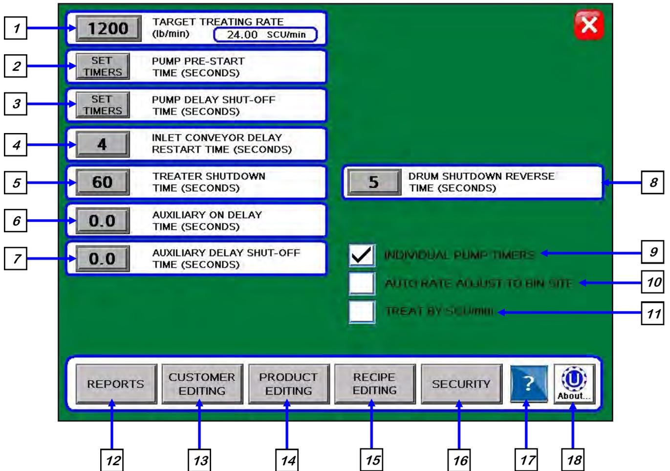
**NOTICE** When buttons 1-7 are pressed, a numeric touch pad (right) will appear allowing the operator to enter in a number for that particular parameter.
