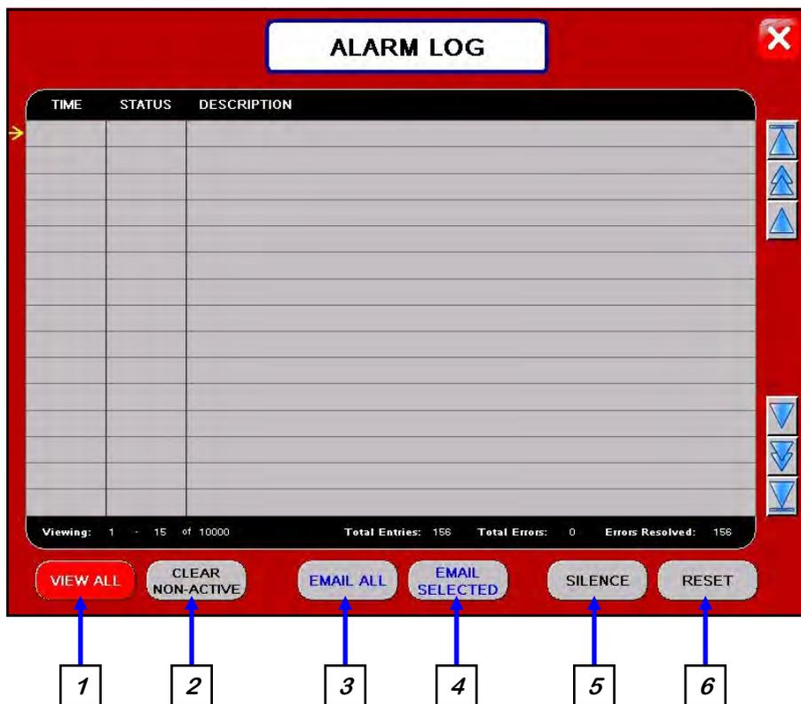
**1. VIEW LIST:** This button toggles between View All to display all alarms and faults stored at any given time (the button will be red) and Hide All which will hide all alarms except the active ones. When an alarm or fault occurs, it will be shown in the list with a red background until the Silence button is pressed, then it will turn yellow.
