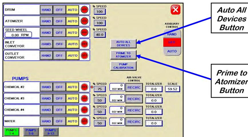
3. Return to the main screen and press the START button. The startup screen appears. Press the gray buttons to change any fields such as customer, seed type and actual weight for this run. Press START to begin the run. The drum, atomizer, inlet conveyor and outlet conveyor will activate. The pump will turn on and re-circulate until it reaches the desired flow rate needed to match the target treating rate that was entered. The inlet conveyor will then begin dumping seed into the seed wheel.
