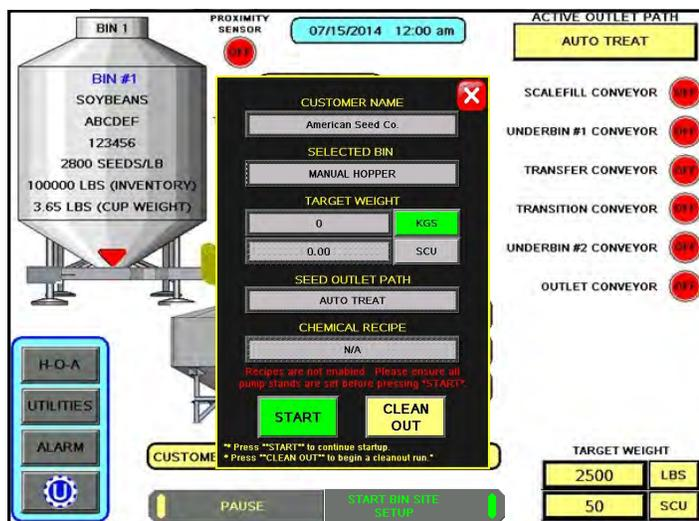
5. Press the SEED OUTLET PATH button, then select either AUTO TREAT or MANUAL TREAT mode of operation depending upon what you plan to do with the seed once it has been pulled from the Pro Box and weighed by the batch hopper system. There may be other names set for different outlet paths an operator may see based on different configuration settings.
