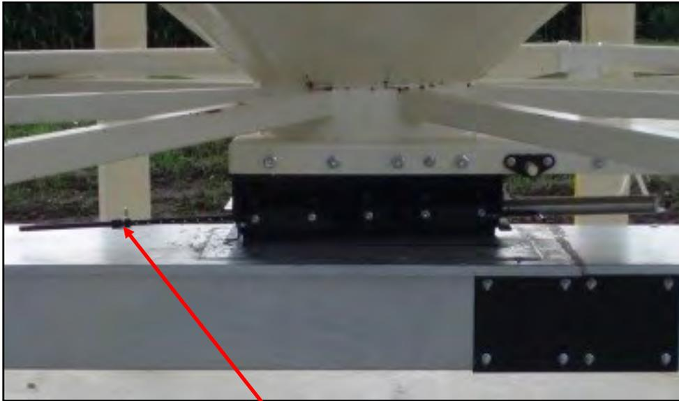
Move the position of the collar along this rod to adjust the flow of seed through the bin slide gate.
