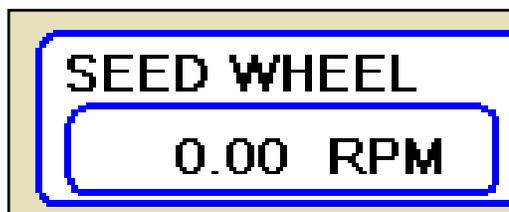
**6. SEED WHEEL PERCENT SPEED:** When this button is pressed, a numeric touch pad (right) will appear to allow the operator to manually adjust the speed of the seed wheel. When running in the AUTO mode the program will override this setting.
