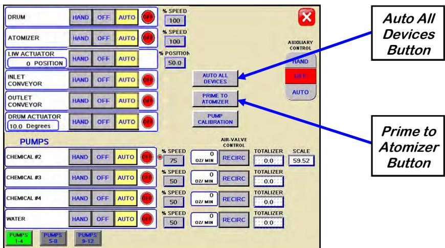
3. Return to the main screen and press the START button. The startup screen appears. Press the gray buttons to change any fields such as customer, seed type and actual weight for this run. Press START to begin the run. The drum, atomizer, and outlet conveyor will activate. The pump will turn on and re-circulate until it reaches the desired flow rate needed to match the target treating rate that was entered.
