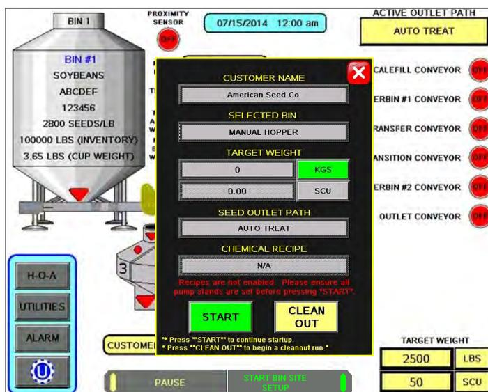
5. Press the SEED OUTLET PATH button, then select either AUTO TREAT or MANUAL TREAT mode of operation depending upon what you plan to do with the seed once it has been pulled from the Pro Box and weighed by the Tri - Flo ® system. There may be other names set for different outlet paths an operator may see based on different configuration settings.
