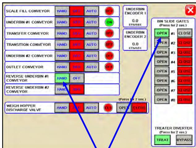
3. Then, manually place the desired bin slide gate to the OPEN position. (top)
