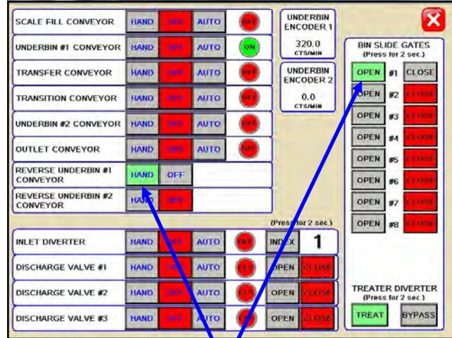
Press the HAND button and then place the bin slide gate to the OPEN position.
