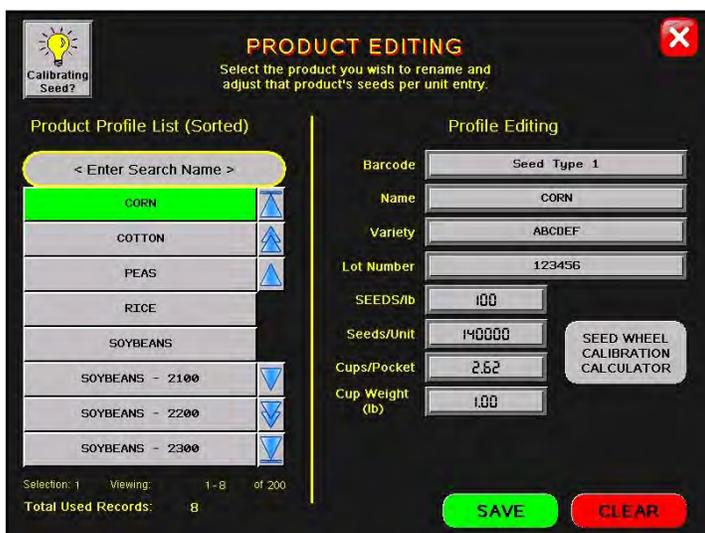
**Note: The seed wheel calibration screen will adjust the seed profiles Cups / Pocket Ratio automatically.**
