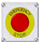
There is an Emergency Stop push button on all LPV and LPX Seed Treaters which is located on the Treater Control Panel. The LPX Automated Treater has an additional Emergency Stop pushbutton on the Main Control Panel. Actuators of emergency stop shall be colored RED. The background immediately around the device actuator shall be colored YELLOW. The actuator pushbutton operated device shall be of the palm or mushroom head type.
