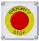
There are three Emergency Stop push buttons. There is one on the Main Control Panel, one on the Tri - Flo™ Control Panel and one on the Bin Site Control Panel. Actuators of emergency stop shall be colored RED. The background immediately around the device actuator shall be colored YELLOW. The actuator pushbutton-operated device shall be of the palm or mushroom head type.
